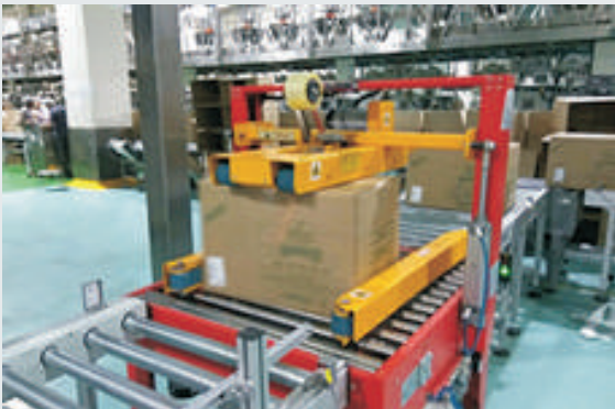
Online auto strapping with Horizontal wrapping Machine
